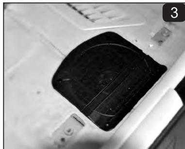
Factory subwoofer is under the cover, ready for the CDT BM8-Sub1 installation.
